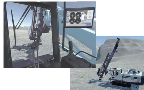
Image displayed on the blast hole drill simulator screen
