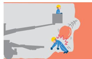
Illustration of collapse near a tunnel face
