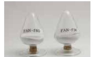
Owing to its excellent thermal conductivity, thermal radiation, and electrical insulation properties, aluminum nitride is a basic material used in semiconductor device fabrication components and substrates.
