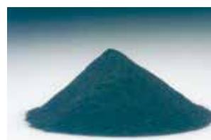
Cupric oxide used for copper plating
