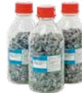
High-purity metallic arsenic—high-purity gallium arsenide semiconductor materials used in mobile phones and other electronic devices, red laser diodes, and LEDs
