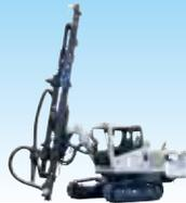
Rock drills (hydraulic breakers, hydraulic crawler drills, tunnel drill jumbos, etc.)
