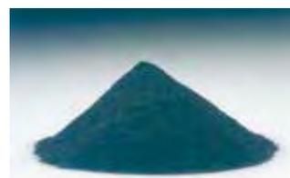
Cupric oxide used for copper plating
