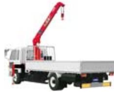
A battery to power the crane and an electric unit that employs proprietary motor control technology have been added to create a new model that allows crane operation when the truck's engine has been switched off. The U-can ECO EV produces zero CO<sub>2</sub> emissions when the crane is in operation\*, and generates considerably less noise.
