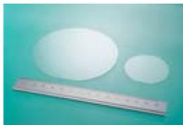
Two-inch GaN substrate and the recently developed four-inch GaN substrate
