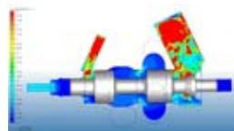
Simulation of the internal flow of a hydraulic drifter
