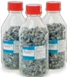
Gallium arsenate semiconductor materials used in cellular phones and other electronic devices, red laser diodes, and LEDs
