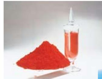
Cuprous oxide is used as an antifouling agent in paints applied to the bottoms of ships.
