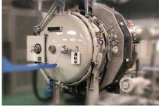
A furnace for manufacturing aluminum nitride ceramics
