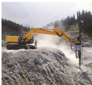
Attachment drill with hydraulic rock drill
