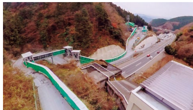
SICON® enclosed hanging belt conveyor adopted for mountain tunnel construction
