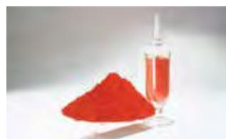
Cuprous oxide is a red powdery substance used to prevent corrosion on the underside of marine vessels.
