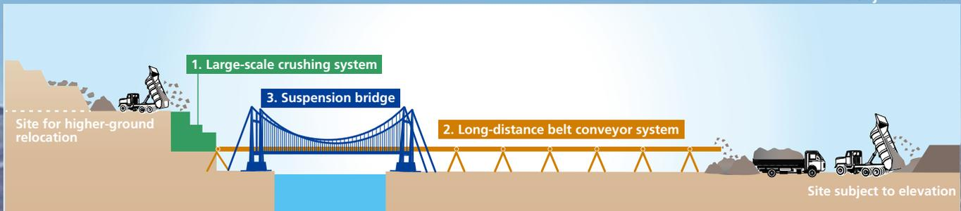
The Group's involvement in the Rikuzentakata City restoration project covers provision of three types of machinery: a large-scale crushing system for crushing earth and gravel, a long-distance belt conveyor system for transporting large volumes of earth and gravel to holding areas, and a suspension bridge for getting materials across a river that lies in between.
