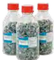
High-purity metallic arsenic—high-purity gallium arsenide semiconductor materials used in mobile phones and other electronic devices, red laser diodes, and LEDs
