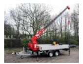
Crane mounted on trailer
